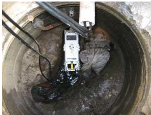
DDS Flo-Dar monitoring flow in 10" line at Allegheny Avenue in Oil City, PA.
