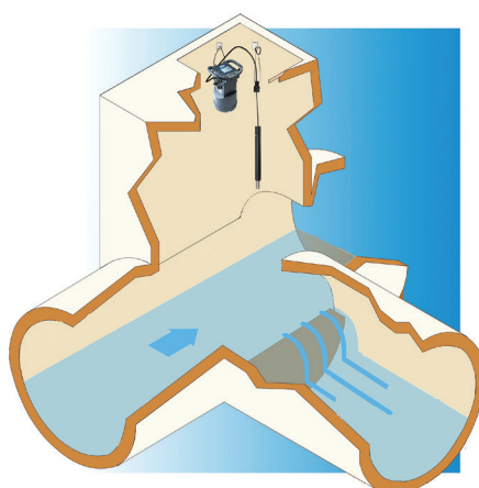
Hach US9001B Ultrasonic Sensor with Ballast
